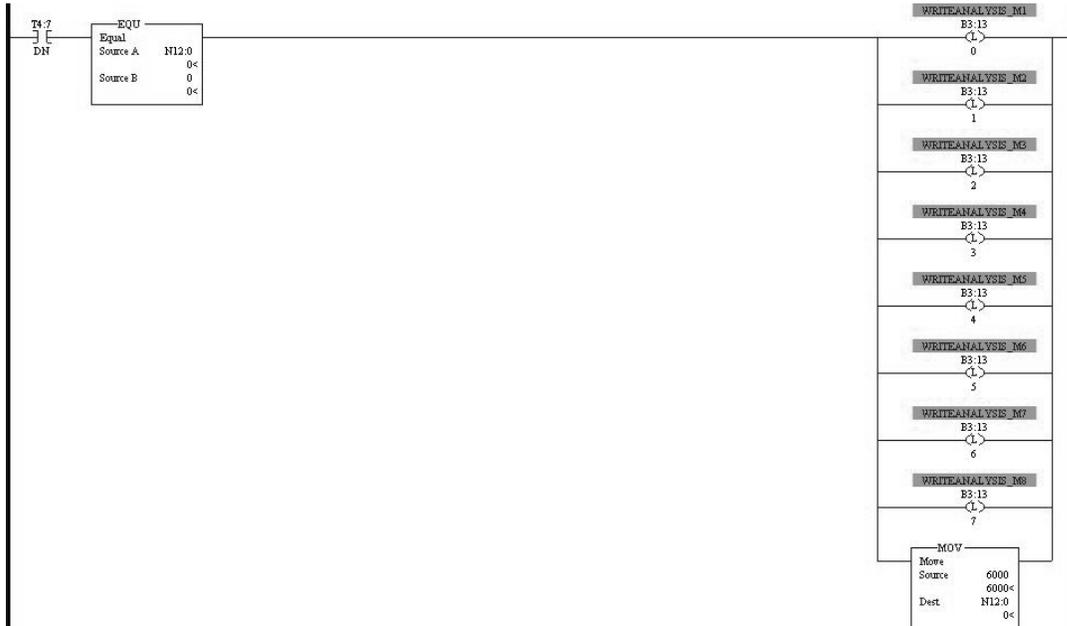
The ladder logic will automatically generate blocks 6000 to 6007 to send the molar analysis data for all meter channels. Some minor modifications may be required depending on each application (for example if some of the meters do not use chromatograph data).
