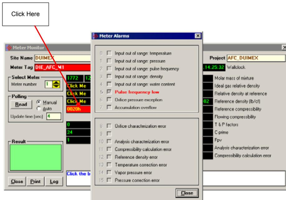
The above image shows the Meter Alarms bitmap, which gives you a quick overview of active alarms. Associated with many of these bits are Alarm Code registers which supply specific reasons for the alarms, most of which appear in the lower right corner of the main Meter Monitor window. For complete information, including which Code registers are associated with which alarm bits, use the Modbus Dictionary feature of AFC Manager.
