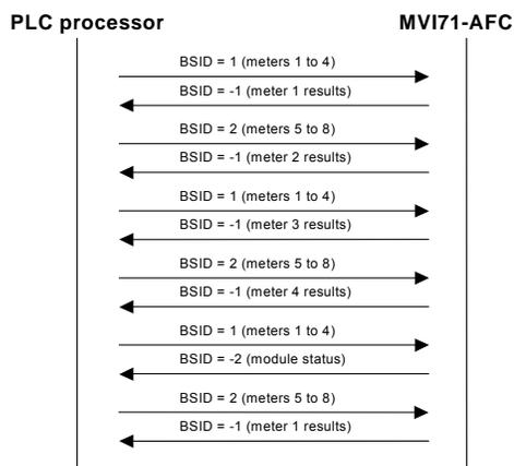
As the diagram shows, the module also periodically sends status blocks (Block Synchronization ID = -2) after every meter cycle.
