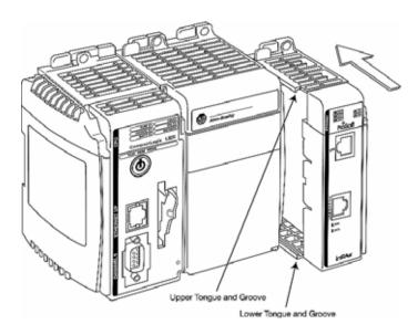
2 Move the module back along the tongue-and-groove slots until the bus connectors on the MVI69 module and the adjacent module line up with each other.
