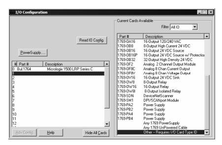
3 On the I/O Configuration dialog box, select "Other - Requires I/O Card Type ID" at the bottom of the list in the right pane, and then double-click to open the Module dialog box.
