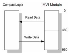
Database address 0 to 479 will be continuously transferred from the module to the processor. Database address 480 to 959 will continuously be transferred from the processor to the module.
