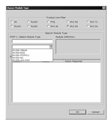
In the Product Line Filter area of the dialog box, select MVI69. In the Select Module Type dropdown list, select MVI69-DNPSNET, and then click OK to save your settings and return to the ProSoft Configuration Builder window.
