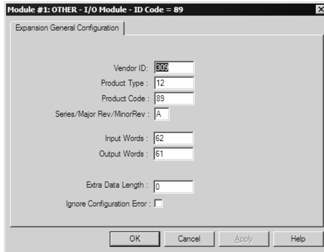
The input words and output words parameter will depend on the Block Transfer Size parameter you specify in the configuration file. Use the values from the following table.
