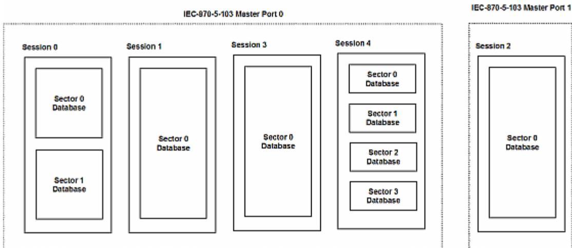
Port 0 on the module communicates with 4 sessions (0, 1, 3 and 4) each of which has their own data set(s). Session 1 only has one sector (all data for device contained in a single database). This sector is addressed by the master using the Common address of ASDU value set for the sector in the configuration file. Session 0 contains two sectors each with their own unique Common address of ASDU value to identify the sector.
