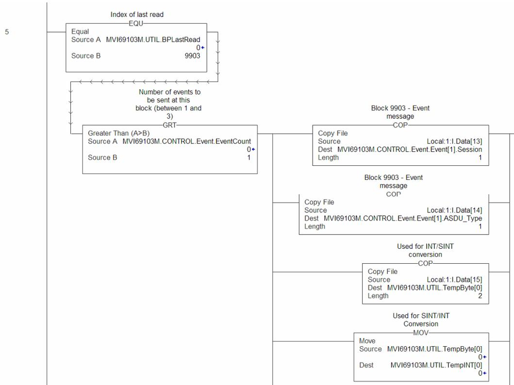
This simple logic does not use the message count parameter in the block and will not work for most applications. It is only provided as an example to display how to move the 9903 data to a user controller tag. If the message pass-through feature is utilized, more logic is required to store the messages received. This feature is most commonly utilized to pass events from the controlled device to an event logger connected to the processor.
