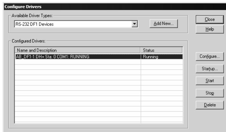
Note: If the list of configured drivers is blank, you must first choose and configure a driver from the Available Driver Types list. The recommended driver type to choose for serial communication with the processor is "RS-232 DF1 Devices".
