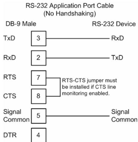
**Note:** If the port is configured with the "Use CTS Line" set to 'Y', then a jumper is required between the RTS and the CTS line on the module connection.
