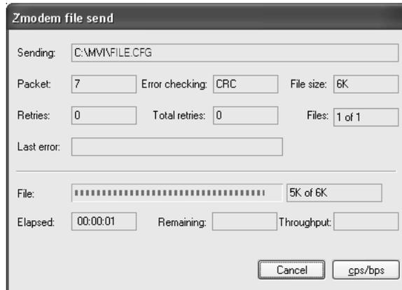
When the upload is complete, the screen indicates that the module has reloaded program values and displays information about the module.
