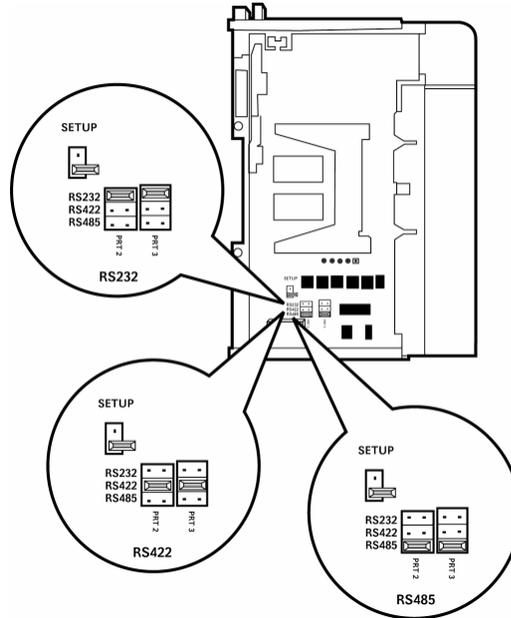
The Setup Jumper acts as "write protection" for the module's flash memory. In "write protected" mode, the Setup pins are not connected, and the module's firmware cannot be overwritten. Do not jumper the Setup pins together unless you are directed to do so by ProSoft Technical Support.
