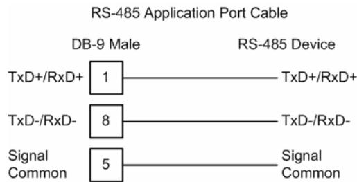
Note: Terminating resistors are generally not required on the RS-485 network, unless you are experiencing communication problems that can be attributed to signal echoes or reflections. In this case, install a 120 ohm terminating resistor on the RS-485 line.
