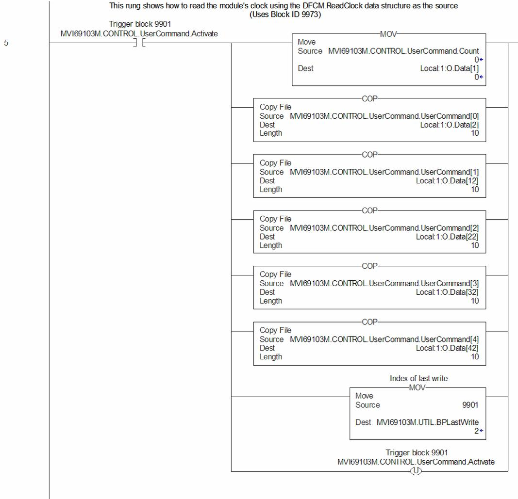
When the command bit (MVI69103M.CONTROL.UserCommand.Activate) is set, the module will build the block 9902 in the output image. The module will receive the new block and place the commands into the command queue for execution.
