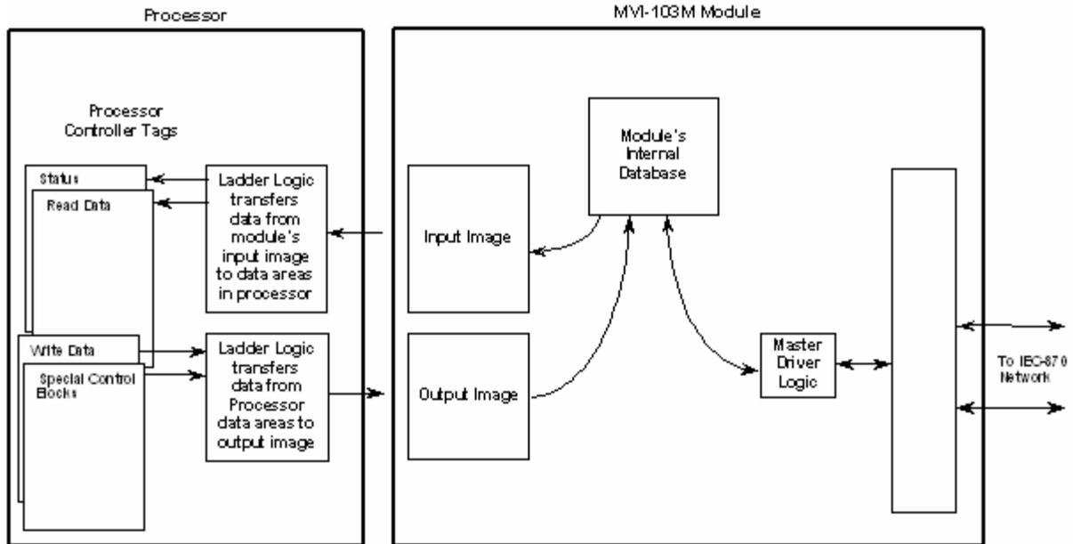
All data transferred between the module and the processor over the backplane is through the input and output images. Ladder logic must be written in the CompactLogix or MicroLogix processor to interface the input and output image data defined in the controller tags. The user is responsible for handling and interpreting all data received on the application ports and transferred to the input image.
