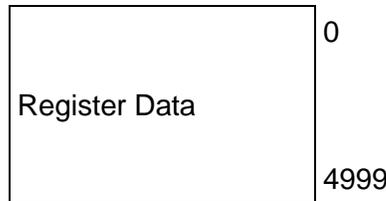
Data contained in this database is paged through the input and output images by coordination of the SLC ladder logic and the MVI46-MNETC module's program. Up to 128 words of data can be transferred between the module and the processor per ladder logic scan. Each image has a defined structure depending on the data content and the function of the data transfer. The following table lists the block numbers used by the module.
