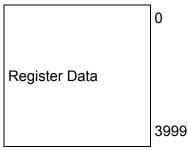
Data contained in this database is constantly updated with the M1 file data by the module and requires no SLC ladder logic to implement. A reserved word in the M1 and database, address 3999, is used as a control register for module control by the ladder logic and for control of the ladder logic by the module.
