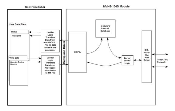
All data transferred between the module and the processor over the backplane is through the M1 file. Ladder logic must be written in the SLC processor to interface the M-file data with data defined in the user-defined data files in the SLC. All data used by the module is stored in its internal database. The following illustration shows the layout of the database:
