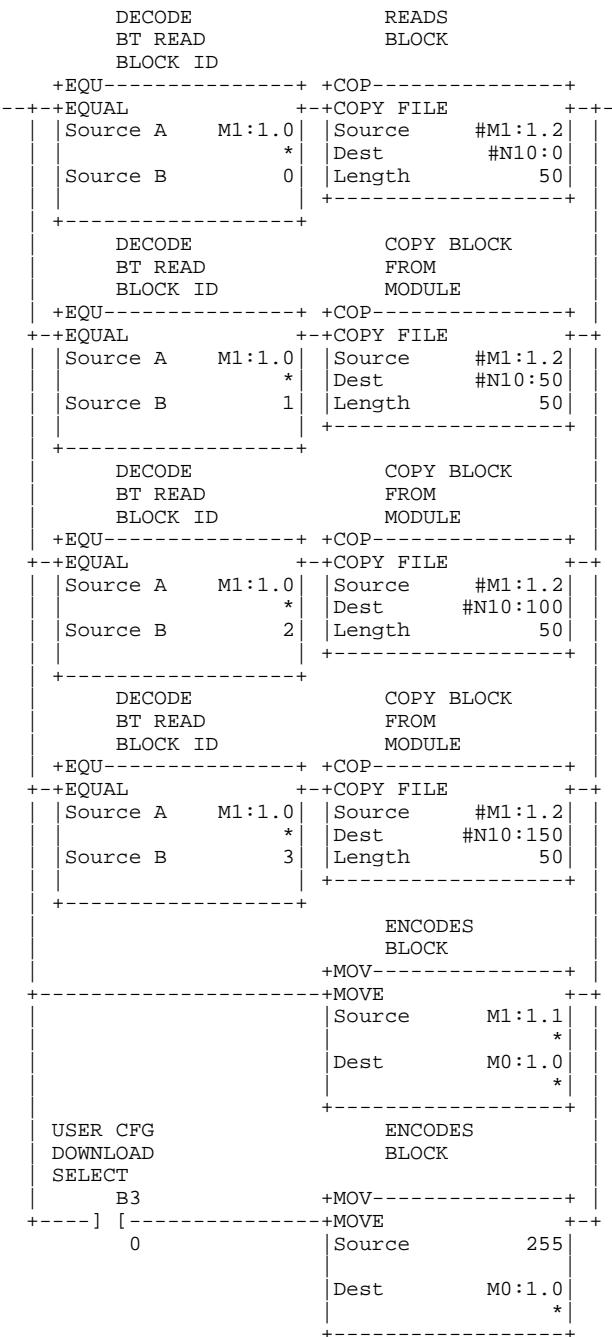
Transfer the BTW Block ID value from the read buffer (word 1) to the write buffer (word 0) to setup the BTW cycle
