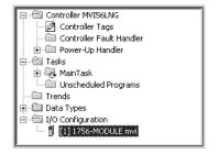
The next step in the module's setup is to define the User Defined Data Types to be used with the module. Copy these data types from the example ladder logic if you are not using the example. They will be defined if you are starting from the example ladder logic. The Controller Organization window should display the User Defined Data Types shown in the following example:
