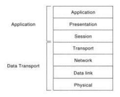
All of the messaging that we are talking about is on the Application layer. We will briefly discuss the connection of EtherNet/IP, however this is not the area of focus here. We are only talking in the reduction of the traffic at the Application layer (shown above).
