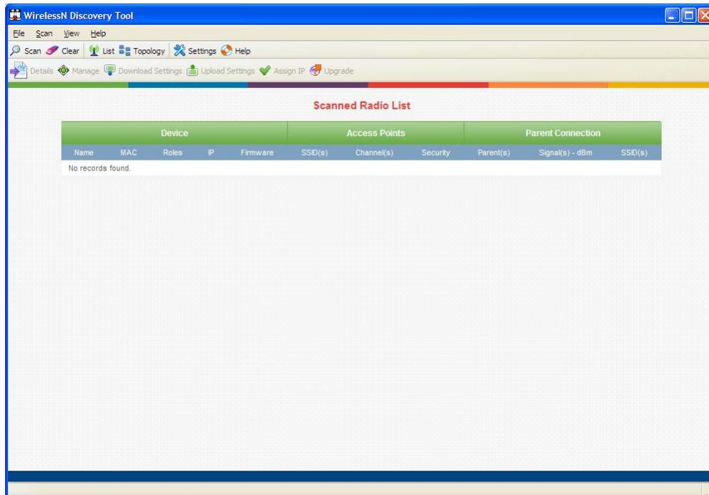
The window lists all the radios your computer can access. The MAC ID number is essentially the serial number of the radio; this number is also printed on the side of the radio. If a radio listing does not appear in the window, click the **SCAN** button. If you still do not see a radio listing, see Troubleshooting in the RLXIB-ICN User Manual.
