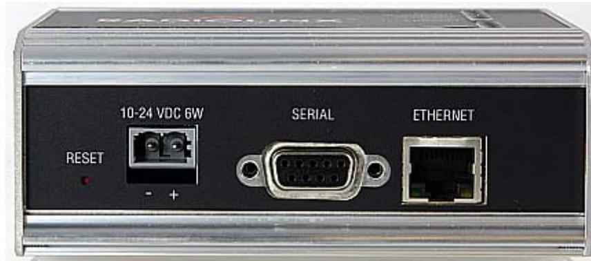
From left to right: Power connector, Serial port, and Ethernet port.
