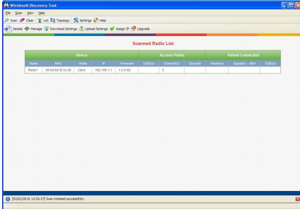
The window lists all the radios your computer can access. The MAC ID number is essentially the serial number of the radio; this number is also printed on the side of the radio. If a radio listing does not appear in the window, click the **SCAN** button on the toolbar. If you still do not see a radio listing, refer to Diagnostics and Troubleshooting in the RLXIB-ICN User Manual.
