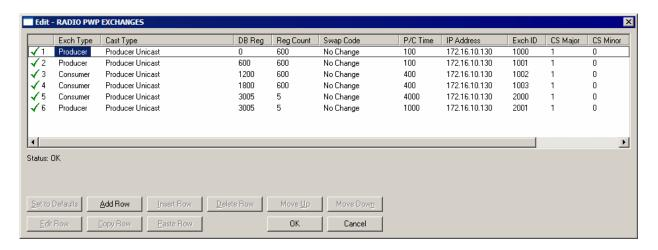
The commands in this section correspond to commands set up in the MNET Client module. For example, the MNET Client module has a Produce command to send data to the MNET Server. The MNET Server must have a corresponding Consume command to match up with the MNET Client Produce command in order to accept the MNET Client produced data.
