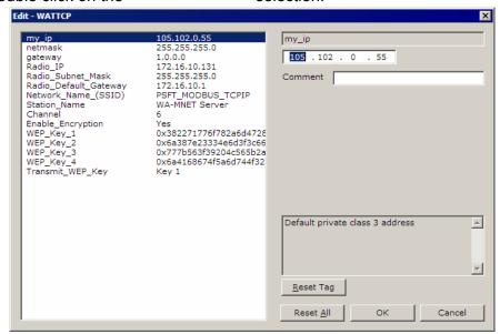
In the sample application, this radio's IP address is set to **172.16.10.131**. In our sample application, the MNET Client IP address is set to 172.16.10.130, so here we used the next IP address in the range which happens to be 131. When you
