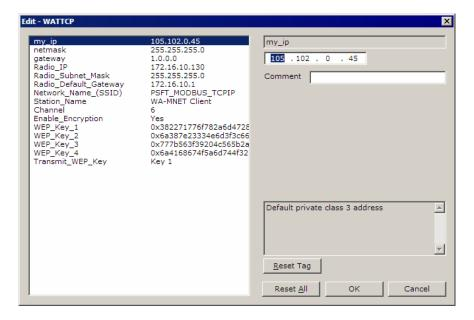
Every Modbus TCP/IP module is set up with the defaults shown in the example. You may have to modify values such as the Radio Default Gateway, the Network Name (SSID), and the Station Name to suit the needs of your network. The Station Name may be modified when using more than one Modbus TCP/IP module.
