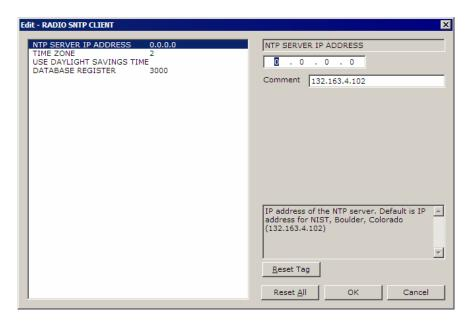
This section is used to synchronize the time using a centralized atomic clock. This feature is only usable if your modules are communicating through an access point such as a RadioLinx Industrial Hotspot. The values in this window should be left with the default values. As you select each parameter, the help window on the screen displays information to help you make your selections. The PWP Driver Manual describes each of these parameters.
