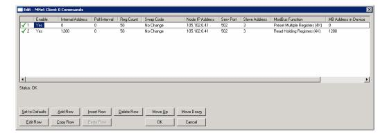
In the sample application, there is one Server device connected to the MNET Client module. The commands in this example show how the data is being written by the MNET Client to the server device, and how the MNET Client is reading the data from the MNET Server device.
