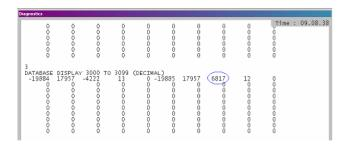
The data shown represents clock values originating from the 6201-WA-MNET Client. The values are stored in 10 registers beginning with register 3000. The clock values are being passed wirelessly to the 6201-WA-MNET ServerThe 6201-WA-MNET Server module is taking this data and passing it back to the 6201-WA-MNET Client and placing it into 5 registers beginning at register 3005.
