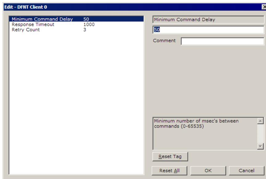
The remaining parameters are set to ensure that the DFNT module can communicate with the Server and with the other client. Refer to the DFNT Driver Manual located on the ProLinx solutions CD for detailed information on each of these parameters.
