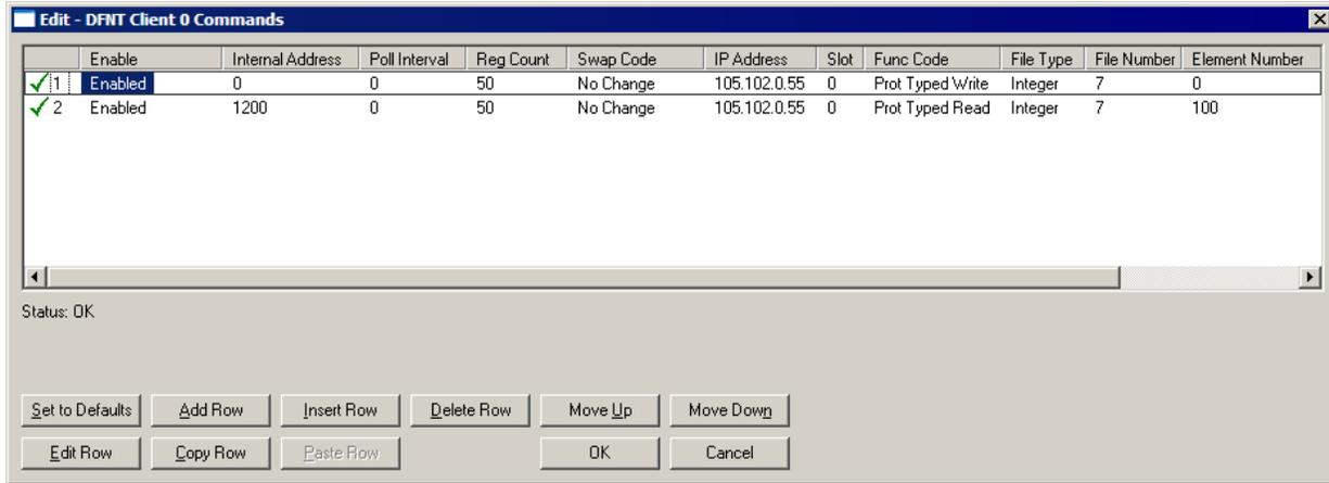
**Note:** For command lines 1 and 2 to function properly with the ControlLogix processor, the menu item "Logic/Map PLC/SLC Messages ..." in the RSLogix 5000 application, must have the "File Number" field in the "PLC 2, 3, 5 / SLC Mapping" dialog box linked / associated with a user specified "Tag Name" Field Tag.
