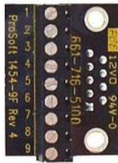
1454-9F DB-9 Female to 9 Pos Screw Terminal adapter (Serial protocol modules only)
