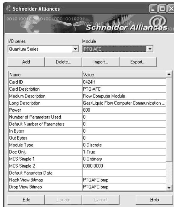
Now you can close the Schneider alliances application and run the Proworx 32 software. At the Traffic Cop section, select the PTQ module to be inserted at the slot:
