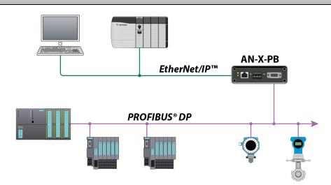
The AN-X3-PB gateway running the HMI firmware acts like a gateway between a PROFIBUS DP network and an Ethernet network supporting EtherNet/IP scheduled connections, PLC5 file emulation, and Modbus TCP.
