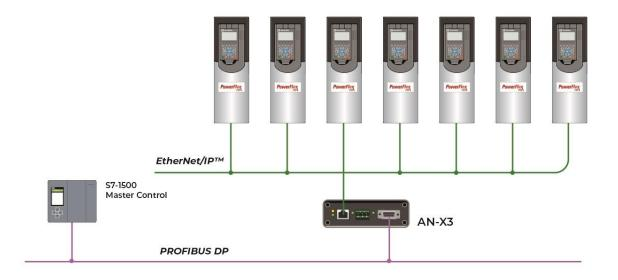
The AN-X3-PB module running AN-X3-PBS-DRV firmware acts as a gateway between a PROFIBUS DP Master and Ethernet/IP motor drives, using Scheduled Connections.
