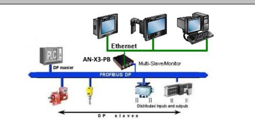
The AN-X3-PB acts as a gateway between a PROFIBUS DP network and an Ethernet network using cyclic UDP messages.
