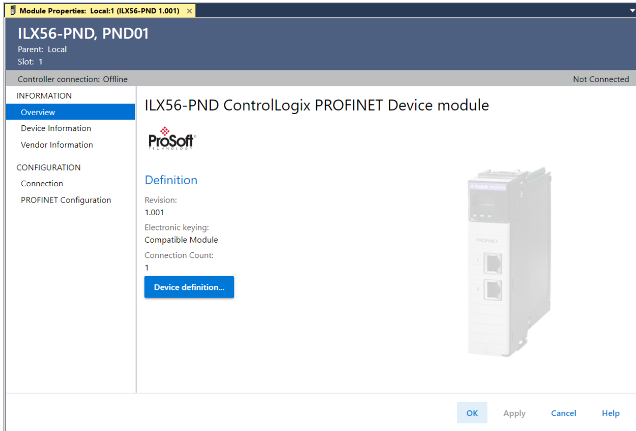
Figure 3.24 – AOP - PLX50 Configuration Utility
