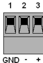
Left to right the pins on the power connector are chassis ground, negative voltage and positive voltage.
