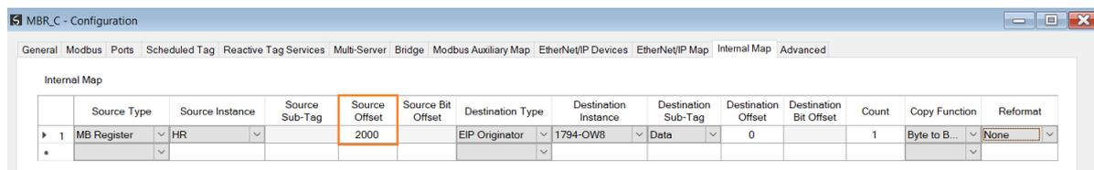
Figure 6.14 – Internal Mapping from Modbus Register to EtherNet/IP IO.
