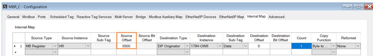
Figure 6.20 – Internal Mapping from Modbus Register to EtherNet/IP.
