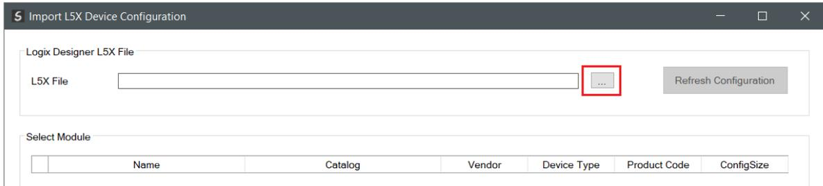
Figure 3.85 – Import L5X Device Configuration – Select L5X.
