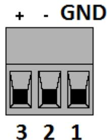
The pins on the power connector are chassis ground, negative voltage and positive voltage. Pin 1 is closest to the Ethernet connector.
