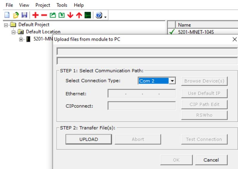
This will upload the configuration from the 5201-MNET-104S module. Now would be a good time to “Save” the PCB file (or .ppf file).
