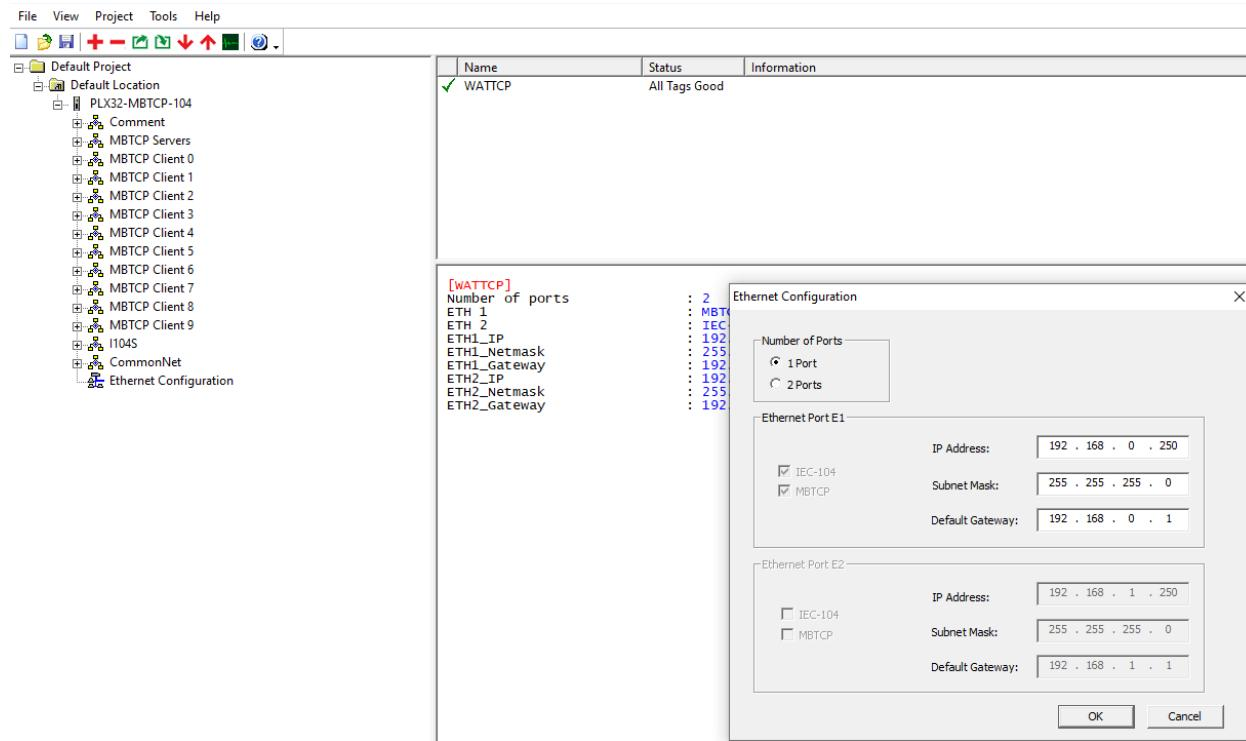
The PLX32-MBTCP-104 module uses this IP address for downloading of the configuration file and diagnostics as well as communication with Ethernet devices. The default IP address of the module is the 192.168.0.250 as shown above.
