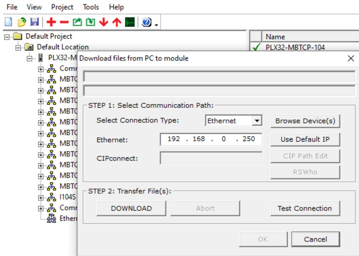
If the module is factory defaults and you are changing the IP address of the module you can select the “Use Default IP” and this will copy the default IP address to the Ethernet settings.
