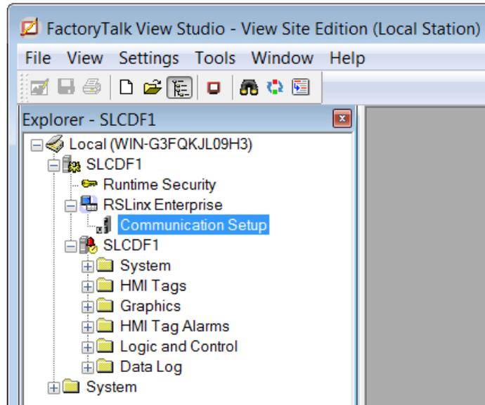
FIGURE 3.30. – FACTORY TALK COMMUNICATION SETUP
