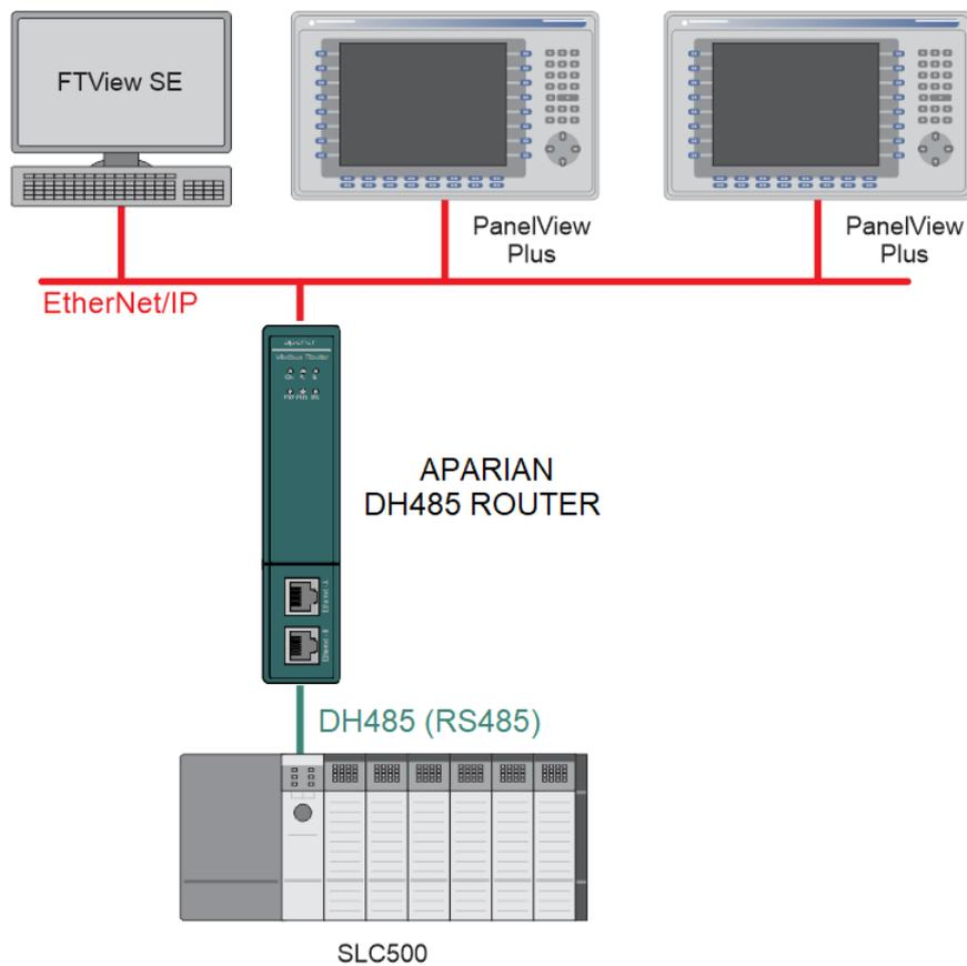
FIGURE 2.1. - EXAMPLE OF A TYPICAL NETWORK SETUP
