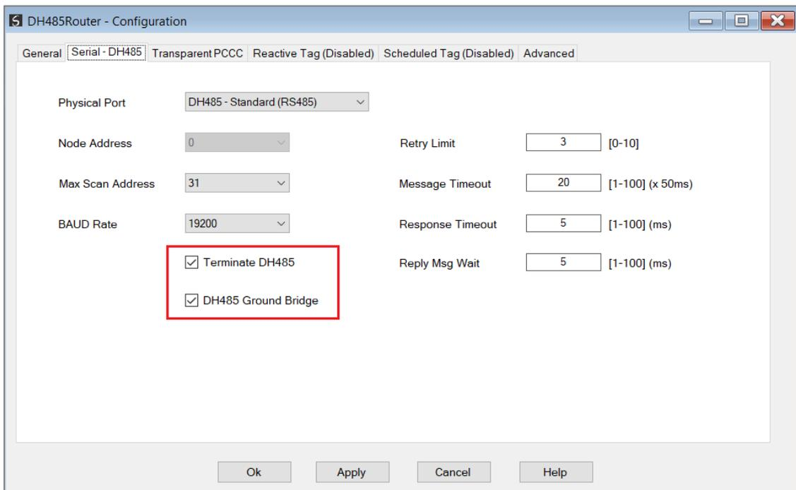
FIGURE 3.7. – INTERNAL RS485 TERMINATION
