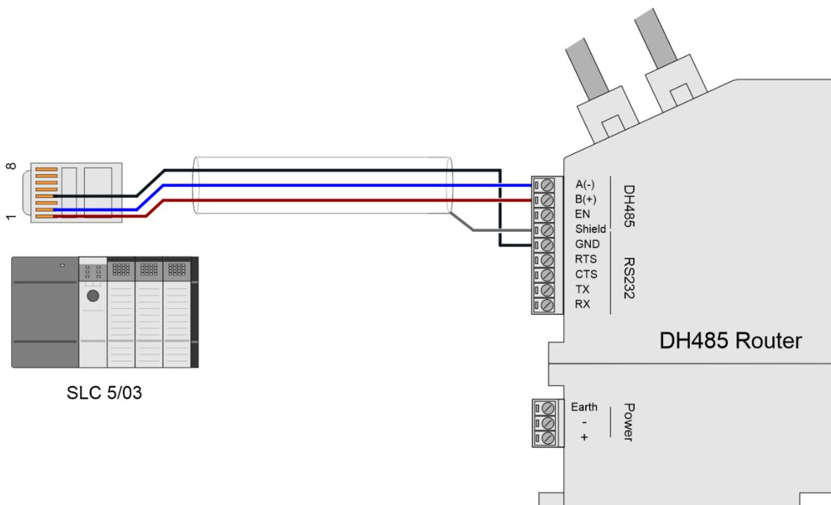
FIGURE 3.3. – SERIAL CABLE PINOUT – SLC DIRECT
