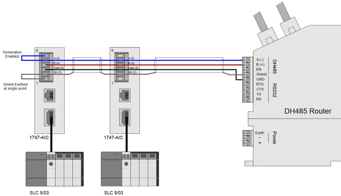
FIGURE 3.2. – SERIAL CABLE PINOUT – 1747-AIC
