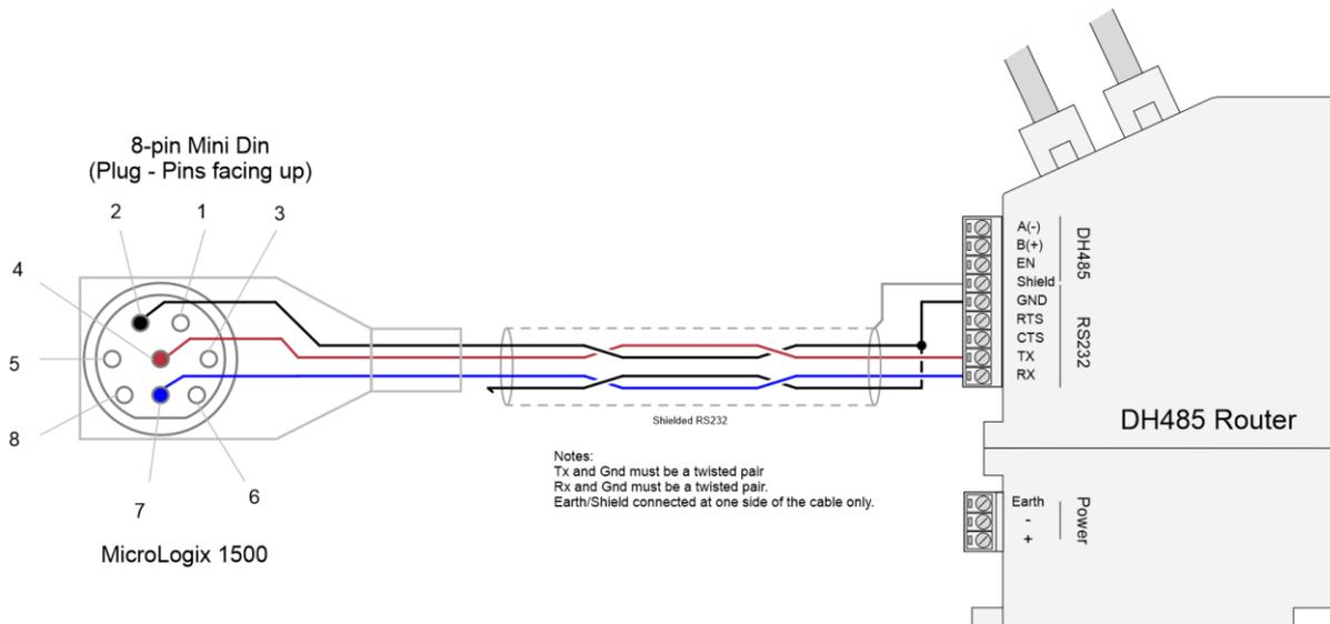
FIGURE 3.6. – SERIAL CABLE PINOUT – MICROLOGIX 1500 (RS232)
