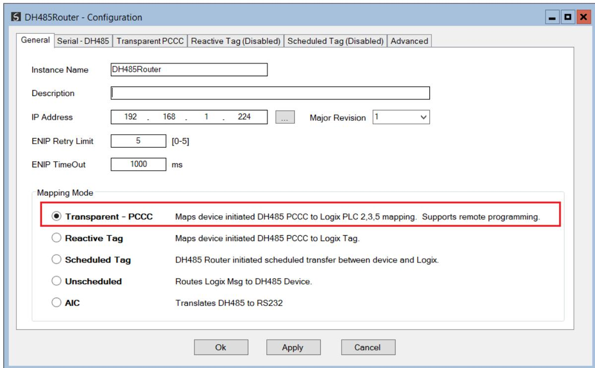
The screenshot shows the 'DH485Router - Configuration' dialog box with the 'General' tab selected. The 'Transparent PCCC' sub-tab is active. The 'Instance Name' is 'DH485Router'. The 'IP Address' is '192 . 168 . 1 . 224'. The 'ENIP Retry Limit' is '5' and the 'ENIP TimeOut' is '1000 ms'. The 'Mapping Mode' section is highlighted with a red box, showing 'Transparent - PCCC' selected. The other options are 'Reactive Tag', 'Scheduled Tag', 'Unscheduled', and 'AIC'.
