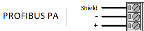
Figure 2.3 – PA Link PROFIBUS PA communications connector
