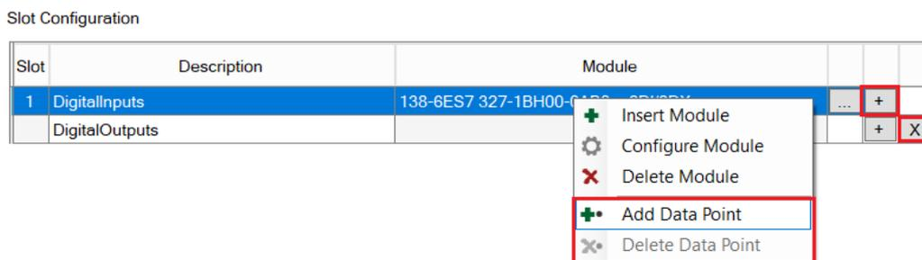
Figure 3.59 – Adding / Removing Data Points
