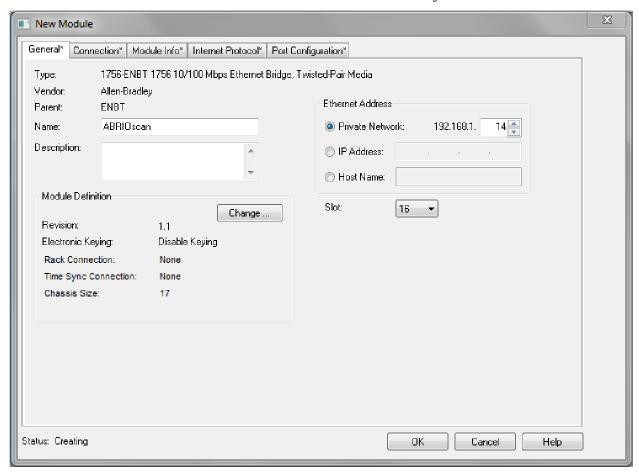
Enter the *Name*. Use the host name you assigned to AN-X when you configured its IP properties.
