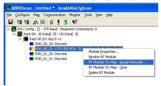
For the inputs and outputs, select the ControlLogix scheduled block and the offset within the block.
