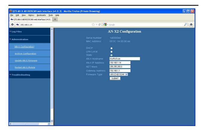
The top of the screen shows the serial number and MAC Address of the AN-X2 being configured.
