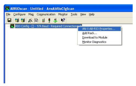
Select *AN-X-ABSCAN Properties* to display the AN-X2-ABSCAN Module Properties dialog box.
