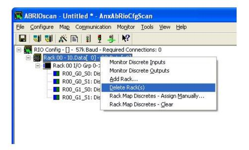
To delete a partial rack, right click on it in the network tree and select *Delete Partial Rack*.
