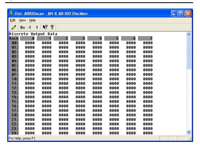
Each row corresponds to a rack. Rack numbers are given in octal. Each row shows the 8 words discrete inputs for the rack number.
