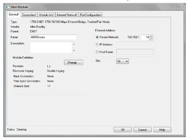
Set the Slot to 16. Set the chassis size to 17.
