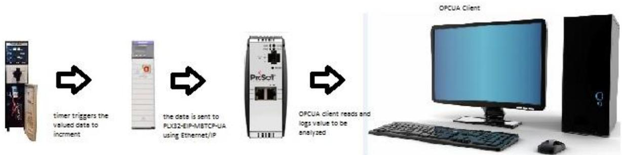
This procedure is performed overnight and the following values are obtained from the logged CSV file using OPC UA Client Application (UAExpert):
